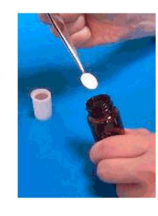
Put filter into vial containing 8 ml of pure water.
