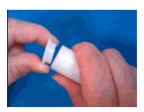
Remove top screen and then exposed filter from sampler using pincers.
