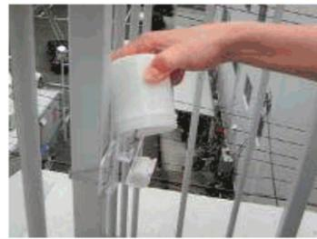
Put exposed passive sampler into brown airtight vial.
