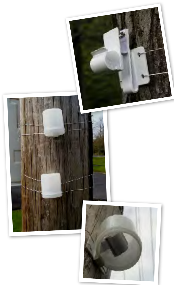
Ogawa Passive Sampler located at outdoor location in Standard Shelter, showing mounting components.
