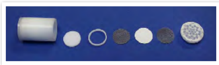
Sampler components (left to right): Body (6), Backing Tab (5), Ring (4), Stainless Steel Screens (2), Collection Pad (3), and Inlet (1).
