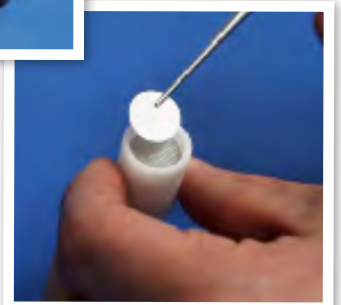
Insertion and removal of Collection Pads is performed using tweezers.
